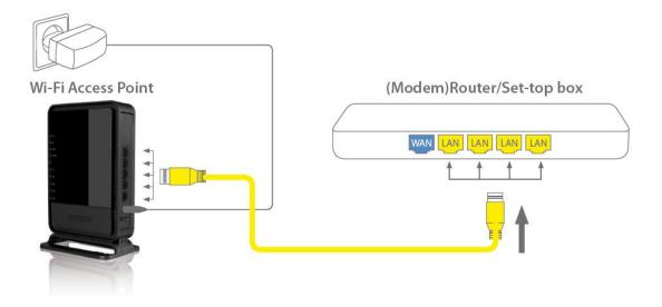
Connect the supplied power-adapter to the power inlet port and connect it to a wall outlet. Switch the access point on by flipping the switch on the back of the device. The access point automatically enters the self-test phase. During self-test phase, the Power LED will be lit continuously to indicate that this product is in normal operation.
